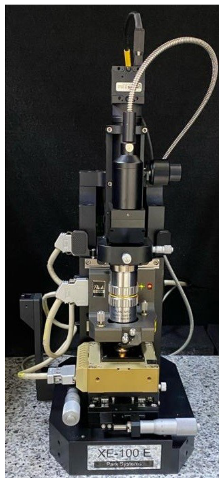
Figure 3. XE-100E atomic force microscope (Park Systems, Suwon, South Korea). The device was used to measure the surface roughness of the tested materials
