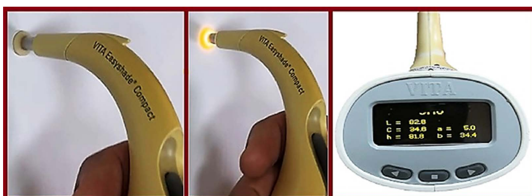
Figure 4. Color measurement using VITA Easyshade
