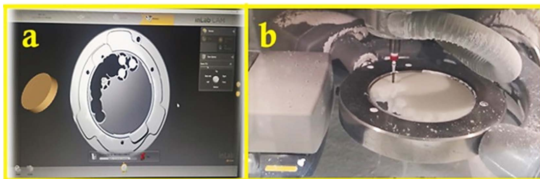
Figure 1. ML zirconia discs fabrication: a) Designing, and b) Milling of ML zirconia discs
